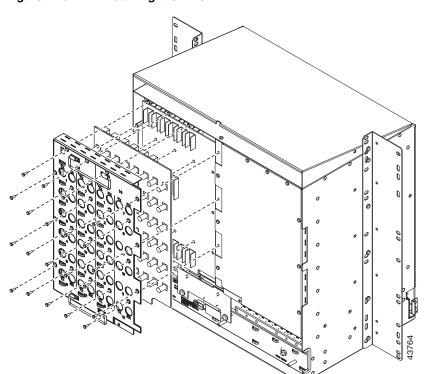
Figure 17-5 Installing the BNC EIA
