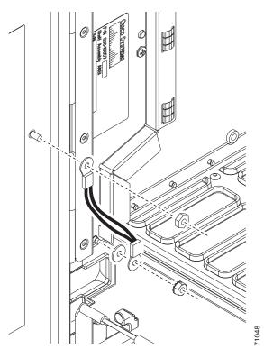
Figure 2-1 Installing the Door Ground Strap Retrofit Kit
