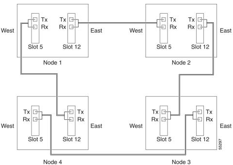
Figure 17-22 shows fiber connections for a four-fiber BLSR. Slot 5 (west) and Slot 12 (east) carry the working traffic. Slot 6 (west) and Slot 13 (east) carry the protect traffic.
