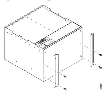
Figure 17-2 Installing the External Brackets
