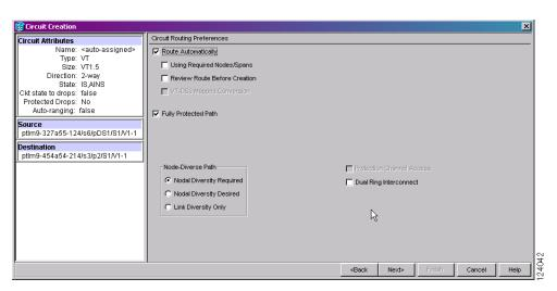
Figure 6-2 Setting Circuit Routing Preferences for a DS-1 Circuit
