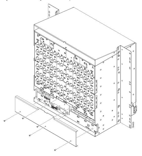
Figure 15-11 Attaching Plastic Lower Backplane Cover
