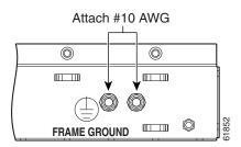
**Step 4** Attach the other end of the shelf ground cable to the equipment bay frame using a dual-hole connector lug per equipment bay frame specifications.
