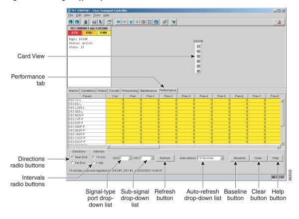
Figure 20-5 Signal Type Drop-Down Lists for a DS3XM-6 Card
