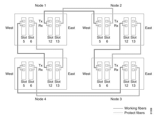
Figure 5-3 Four-Node, Four-Fiber BLSR Fiber Connection Example
