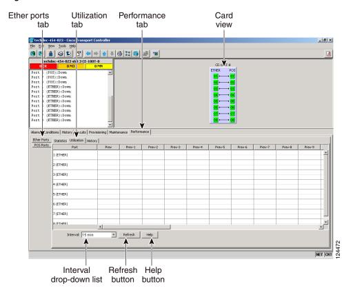
Figure 20-18 Ether Ports Utilization on the CE-Series Card View Performance Window
