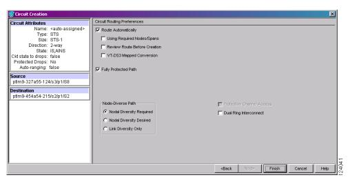
Figure 6-10 Setting Circuit Routing Preferences for an Optical Circuit
