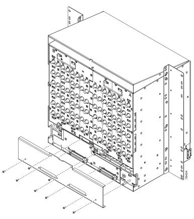
Figure 1-5 Installing the AEP Cover
