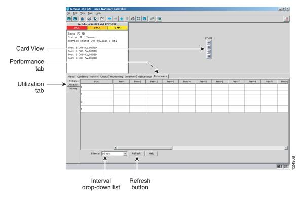
Figure 20-7 FC\_MR-4 Utilization on the Card View Performance Window
