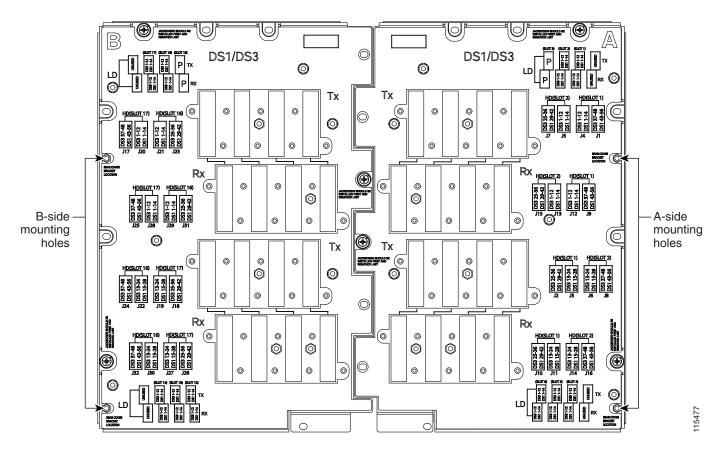
Figure 1-9 Mounting Holes on the UBIC-H
