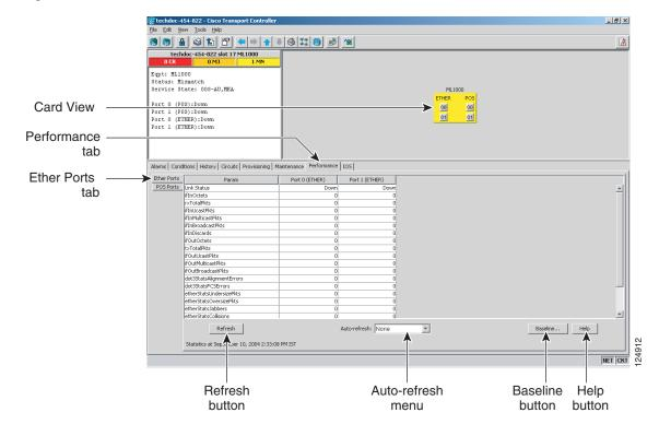
Figure 20-1 Ether Ports on the ML-Series Card View Performance Window
