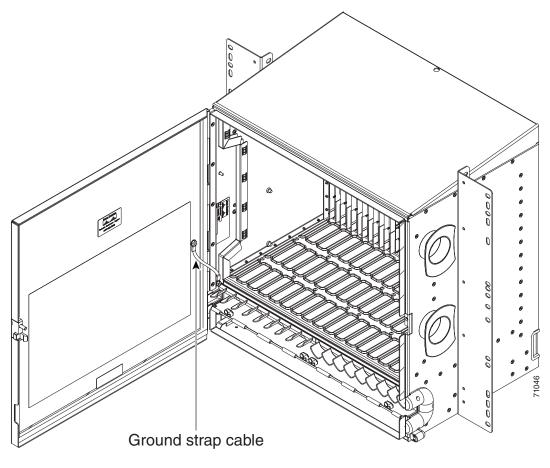
Figure 2-2 Shelf Assembly with Door Ground Strap Retrofit Kit Installed
