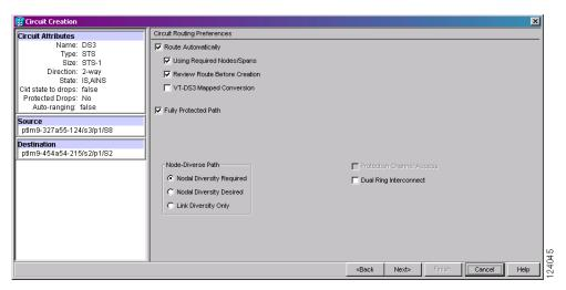
Figure 6-5 Setting Circuit Routing Preferences for a DS-3 or EC-1 Circuit
