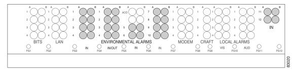
Figure 17-13 shows alarm pin assignments in a shelf for Release 3.3 and earlier. The AIC-I is incompatible with shelves Release 3.3 or earlier.
