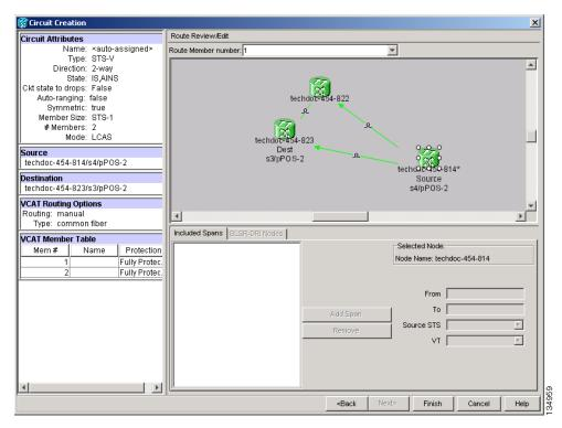
Figure 20-3 Manually Routing a VCAT Circuit
