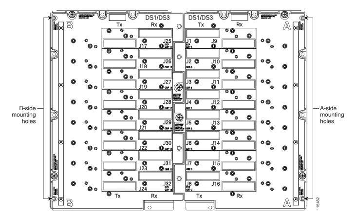
Figure 1-10 Mounting Holes on All Other EIA Types
