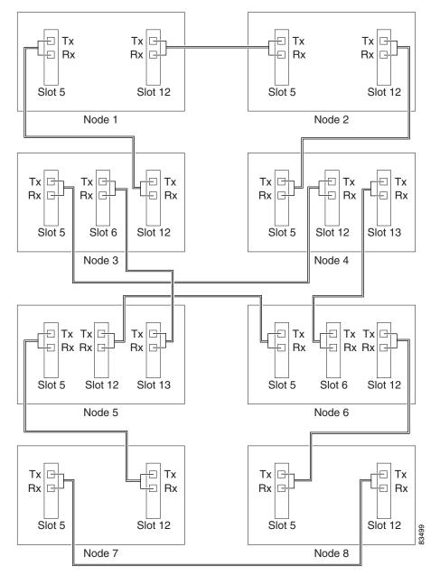
Figure 17-19 Connecting Fiber to an Eight-Node Traditional Path Protection Dual-Ring Interconnect
