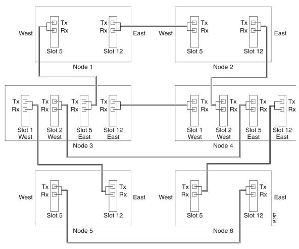
Figure 5-5 Integrated Two-Fiber BLSR DRI Example
