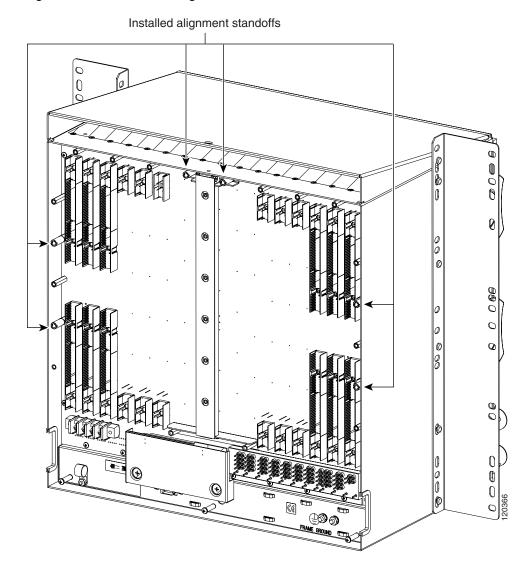
Step 6 Line up the alignment pins on the UBIC-H EIA (Figure 20-23) with the alignment standoffs on the shelf and push the UBIC-H EIA with consistent pressure until the pins and standoffs fit together firmly.
