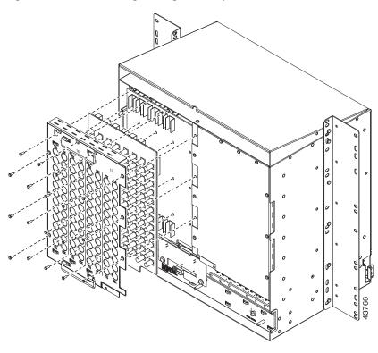
Figure 17-6 Installing the High-Density BNC EIA
