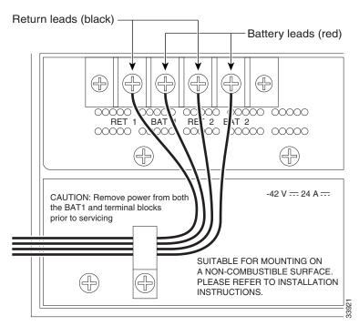
Remove or loosen the #8 power terminal screws on the ONS 15454. To avoid confusion, label the cables Step 4 connected to the BAT1/RET1 (A) power terminals as 1, and the cables connected to the BAT2/RET2 (B) power terminals as 2.
