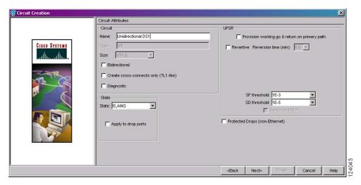
Figure 6-3 Setting Circuit Attributes for a Unidirectional DS-1 Circuit
