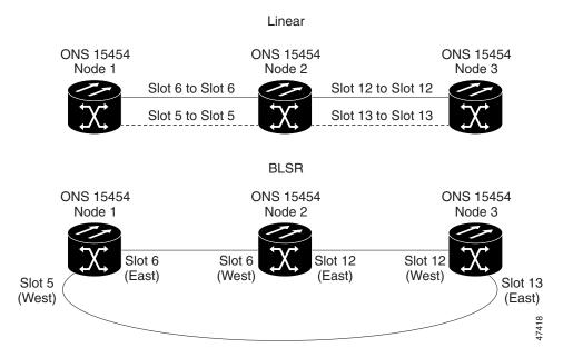
**Step 10** Create the ring by connecting the protect fiber from one end node to the protect port on the other end node. For example, the fiber between Node 1/Slot 5 and Node 2/Slot 5 (as shown in Figure 13-3) can be rerouted to connect Node 1/Slot 5 to Node 3/Slot 13.
