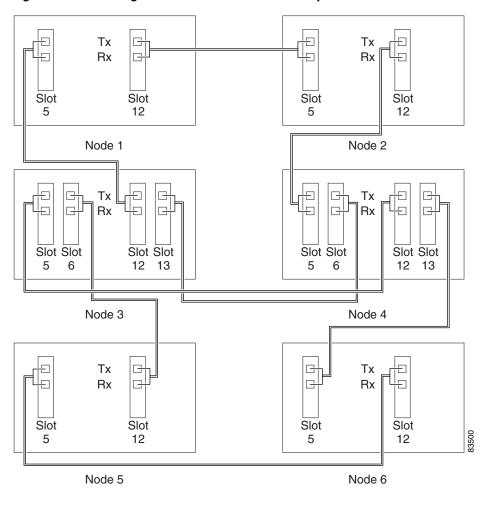
Figure 5-8 Integrated Path Protection DRI Example
