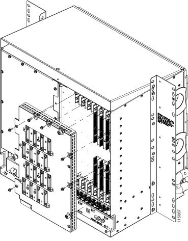
Figure 18-10 Installing the UBIC-V EIA
