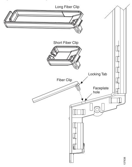
Figure 21-3 Installing the Fiber Clip
