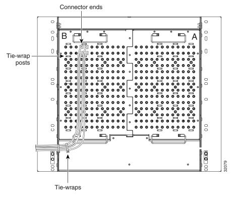
Figure 17-17 Routing Coaxial Cable (SMB EIA Backplane)
