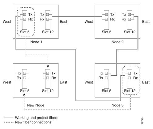
Figure 14-1 Three-Node, Two-Fiber BLSR Before a Fourth Node Is Added
