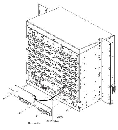
Figure 1-3 Installing Standoffs and the AEP
