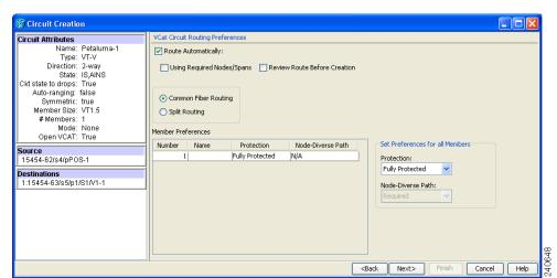
Figure 6-16 Automatically Routing a VCAT Circuit
