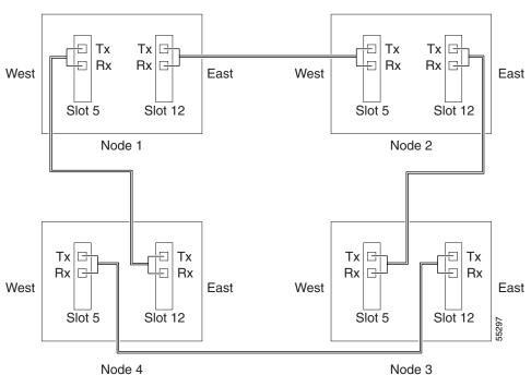
Figure 5-2 Four-Node, Two-Fiber BLSR Fiber Connection Example
