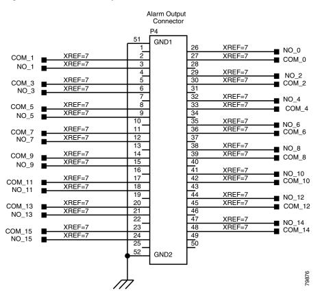
Figure 1-7 Alarm Output Connector
