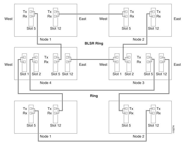
Figure 5-10 Integrated BLSR to Path Protection DRI Example
