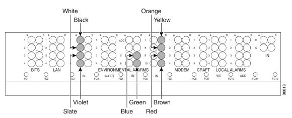
Figure 1-4 AEP Wire-Wrap Connections to Backplane Pins
