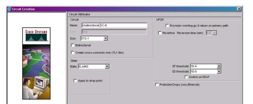
Figure 6-11 Setting Circuit Attributes for a Unidirectional Optical Circuit
