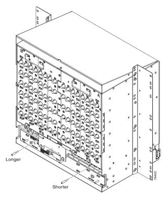
Figure 1-2 Replace Backplane Screws with Standoffs
