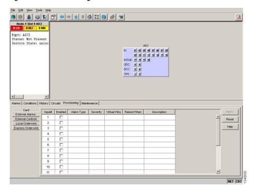
Figure 8-3 Provisioning External Alarms on The AIC-I Card
