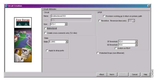
Figure 6-6 Setting Circuit Attributes for a Unidirectional DS-3 or EC-1 Circuit
