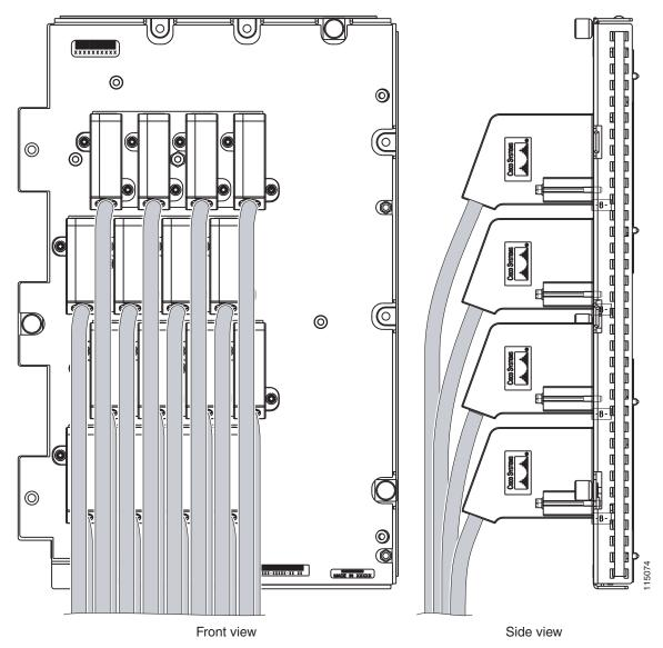
Figure 20-15 Fully Cabled UBIC-V; Front- and Side-View
