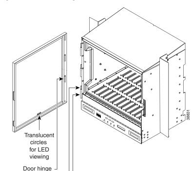
Figure 17-4 Removing the ONS 15454 Front Door
