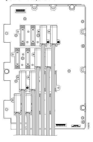
Figure 20-16 Partially Cabled UBIC-V
